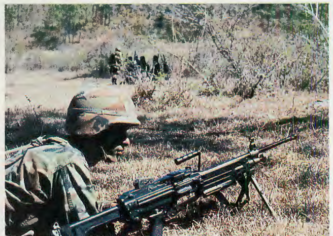
BELOW: Trooper with new M249 SAW (Squad Automatic Weapon), our version of the Belgian FN Minimi. With a full box of 200 belted rounds, the M249 weighs less than an empty M60. A belt cannister attaches firmly to the weapon, helpful for assault fire, and standard M16 magazines can also be used.
